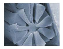
Effective noise reduction is required for optimal acoustics in state-of-the-art automobiles. For tiers and OEMs we offer solutions based on our innovative proprietary Evolon technology. This enables us to produce filaments up to 100 times thinner than human hair which are ideally suited to absorb noise.
