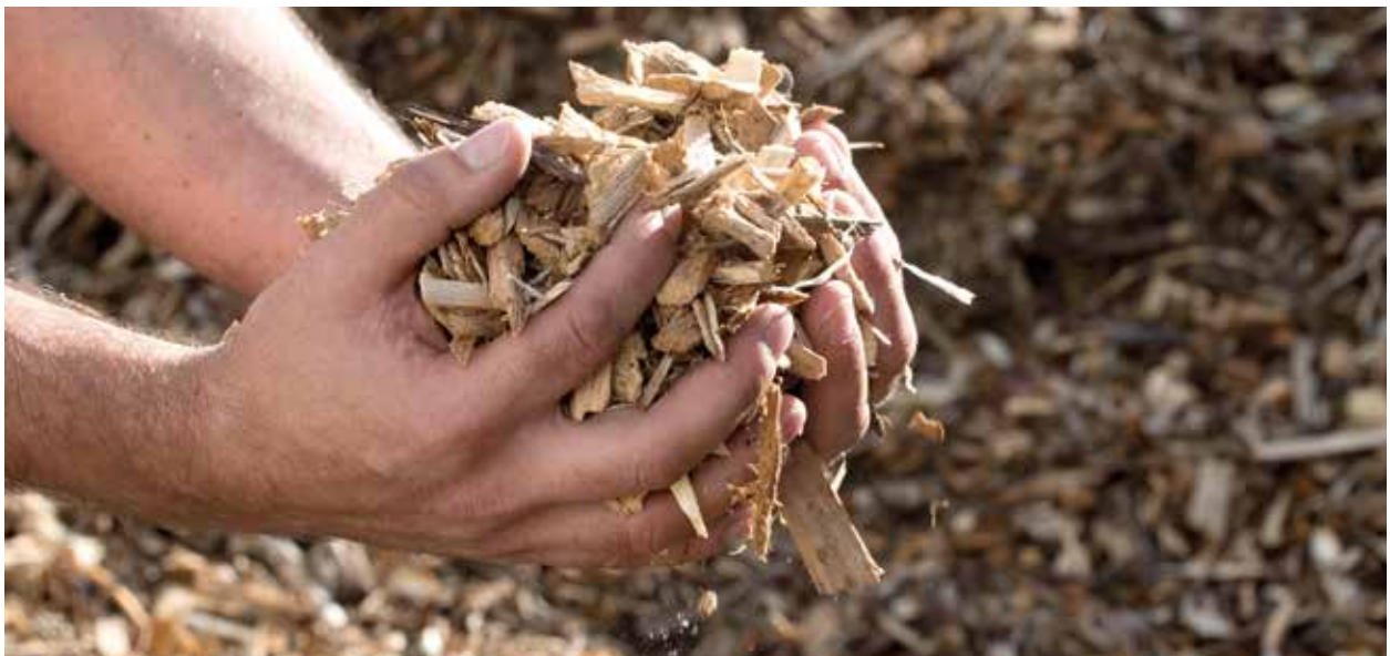
Heating industrial buildings with woodchips as fuel: A good idea when the raw material is available as a waste product of the local wood industry.
